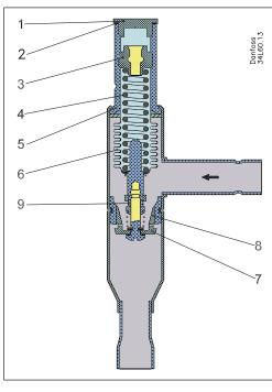
The hot gas bypass regulator KVC opens at a fall in pressure on the outlet side, i.e. when the pressure in the evaporator is beyond the set value.
