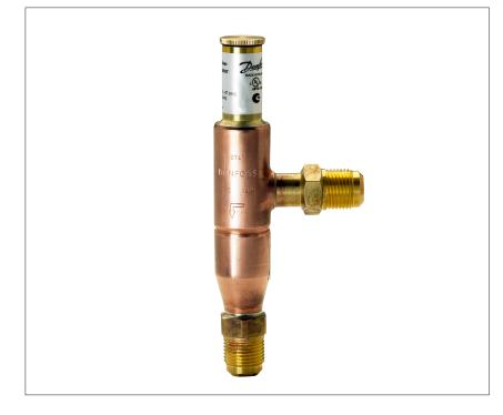
KVC is a hot gas bypass regulator applied for the adaption of the compressor capacity to the actual evaporator load. Placed in a bypass between high and low
